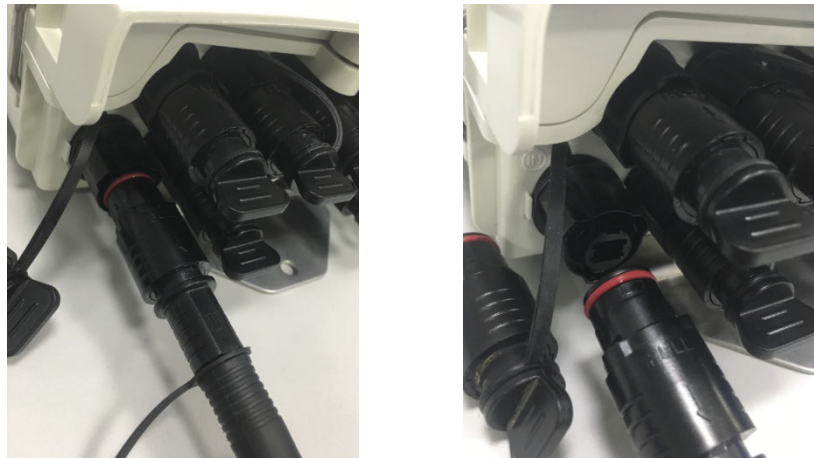
Pic7 Insert and Pull out the fiber connector
