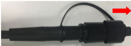
Pic 7 Remove the fiber connector cap and remove the ceramic ferrule cap
