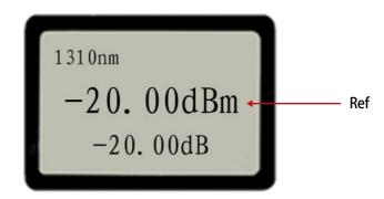
In order to get the loss between the two measurements, do another time testing under the first relative output power. The relative value will be calculated automatically. For example the second time testing of 1310nm output power is -35dBm, the relative output power will be -15dBm. (relative output power=absolute output power-reference value -15dBm=-35.00dBm-(-20.00dBm) see as following:
