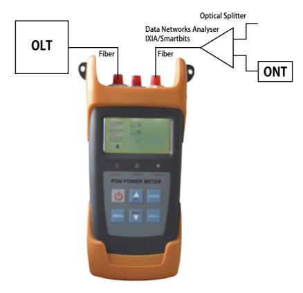
OLT PON Interface optical power test configuration diagram
