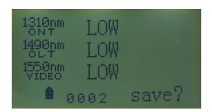
Press "Interest", there will displaying saving on the screen, check with the upper pic. The data recording series No.is 0002. press "Interest" saving, and "Interest" for cancel, and the saving recording can be checked in the "data view" under "historical data" Menu.
