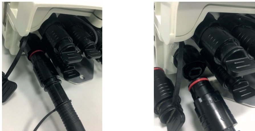
Pic 8 Insert and Pull out the fiber connector
