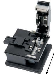
3. After close cover plate, ensure that the fiber is in a horizontal line.
