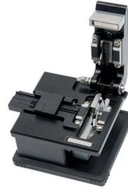
2. Push to the front of the cutting slider(-Figure), press and close the pressure fiberboard and cover plate to fix optical fiber
