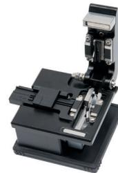
6. After finish cutting, please clean up the broken fiber and don't damage blade for later use.
