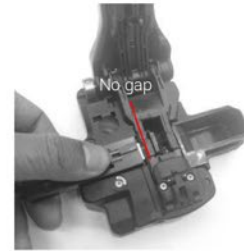
8. Using fiber cleaver cut off bare fiber.
