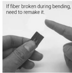
6. Bending fiber(>60°) in 4 directions and a least 3 times to do fiber screening to check if any fiber broken.
