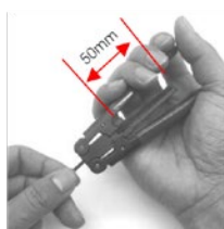
1, Mark 50mm using cable stripper remove outer jacket.
