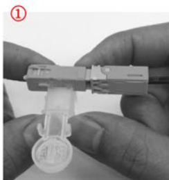
1. Using dust cap into two slots on SC shell.
