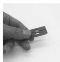
3, Put cable clamp onto the black jig.
