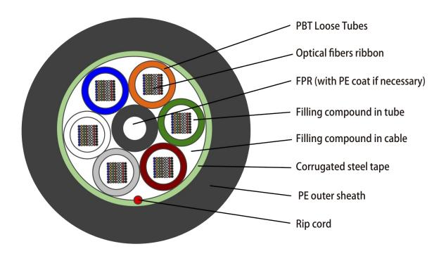
Schematic for reference only. Structure of other fibre counts refer to 3.4.
